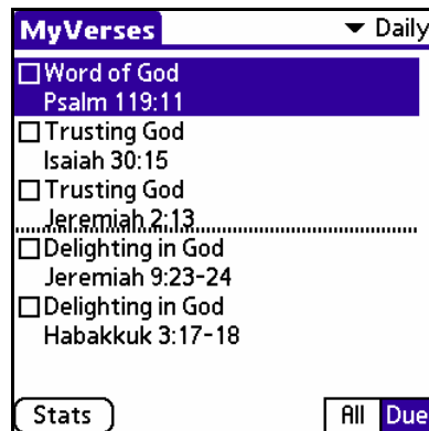
Figure 12-2 Drag the stylus, while maintaining contact with the screen, until the dotted line is at the desired location.
