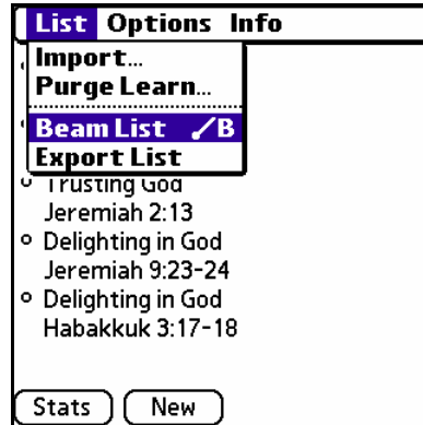
Figure 3-13 Entire lists may be beamed by selecting Beam List from the List menu on the List form.
